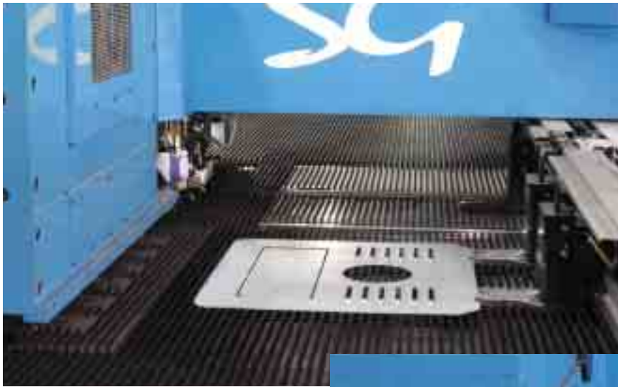
Last-part unload from a shear-and-punch machine using no trim strip. The third clamp moves, then the machine trims the last part with the punch rather than the shear for maximum sheet utilization.
