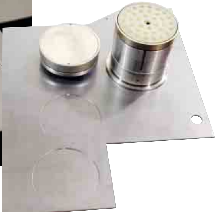
Pacific Energy creates 4.125-in.-dia. knockouts in 0.062-in. hot-rolled steel using upform stations (tools are seen in the photo below) on its shear-and-punch machines.
