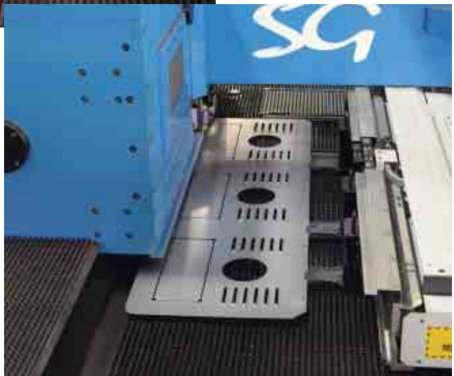
Last-part unload from a shear-and-punch machine using no trim strip. The third clamp moves, then the machine trims the last part with the punch rather than the shear for maximum sheet utilization.
