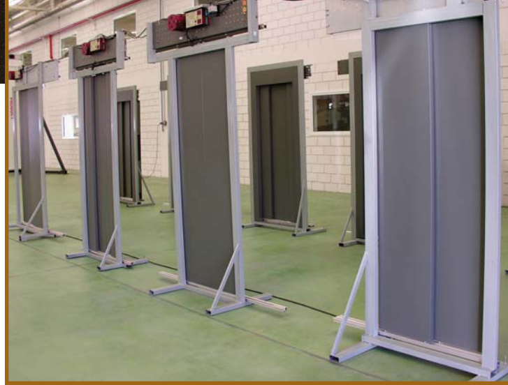
Automated doors that are produced at Tecnoamérica are put through rigorous testing to ensure the highest quality and safety.
