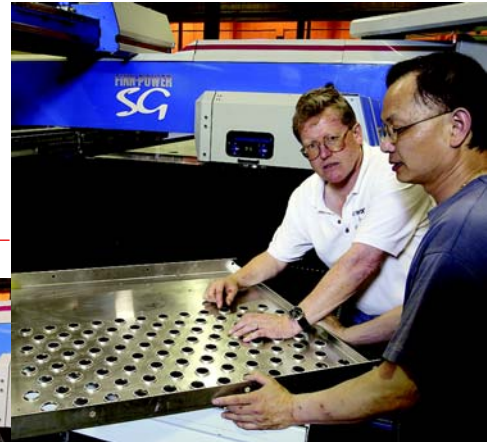
This refrigeration access door assembly is punched, sheared, and ribbed with the Aero-Heat logo on the Shear Genius 6.4 FMC.
