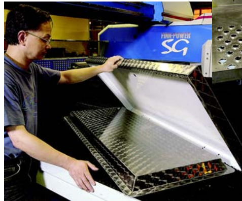
This refrigeration access door assembly is punched, sheared, and ribbed with the Aero-Heat logo on the Shear Genius 6.4 FMC.
