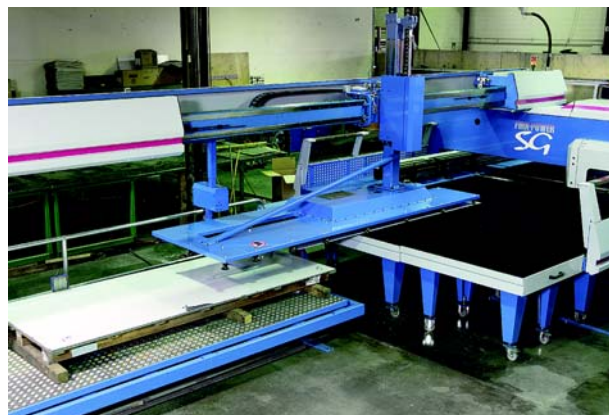
Shear Genius eliminates the potential for mistakes when manually shearing a 60" x 144" sheet as the sheet is loaded and square automatically without human intervention.
