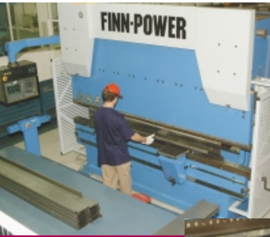
Semeato recently purchased a Finn-Power 160 ton, 4 axis hydraulic press brake. The Finn-Power hydraulic press brake is designed for high precision performance in the most demanding applications.
