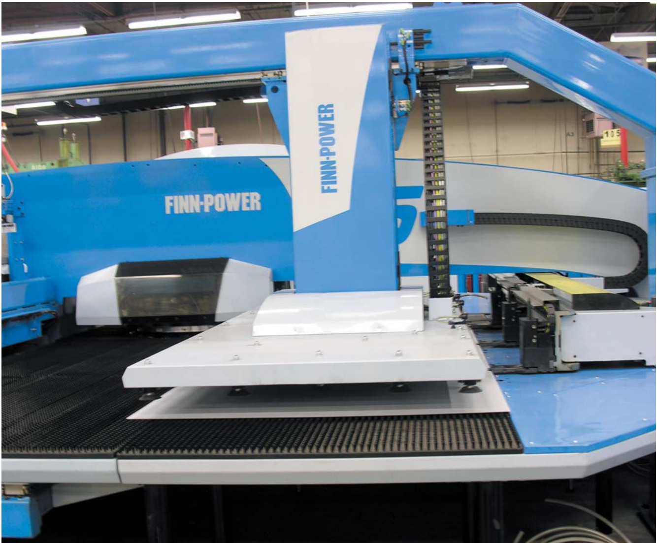
The Finn Power C5 Compact Express provides highly compact load/unload automation by utilizing the space above and below the turret punch press.
