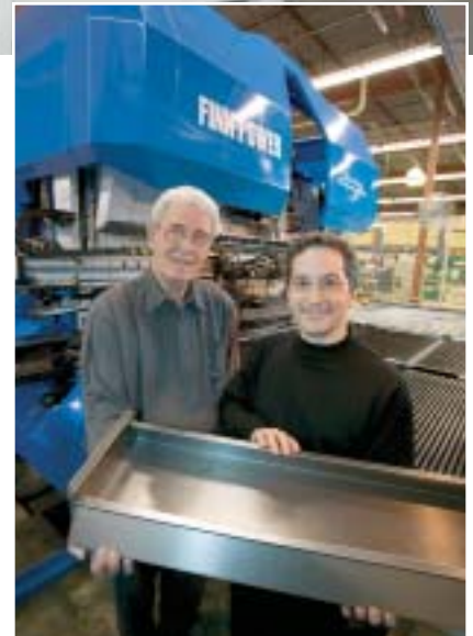
Automated loading and complex bending of light-fixture bodies is a reality at Peerless courtesy of this machine, a Finn-Power Express Bender. Its capability is exhibited in the fixture body held by Marcel Reweghs (left), Peerless operations manager, and Barry Fagen, vice president.
