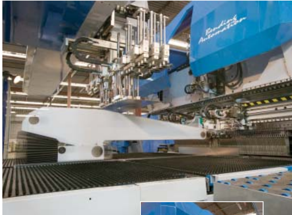
Automated loading and complex bending of light-fixture bodies is a reality at Peerless courtesy of this machine, a Finn-Power Express Bender. Its capability is exhibited in the fixture body held by Marcel Reweghs (left), Peerless operations manager, and Barry Fagen, vice president.
