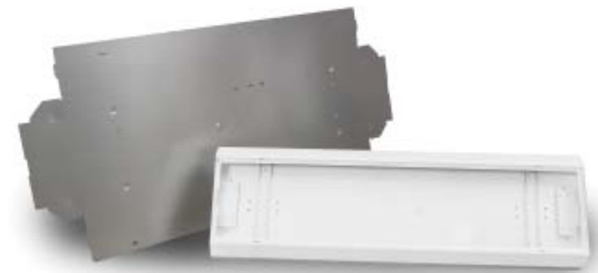
The combination turret press and right-angle shear provides a finished blank that undergoes press-brake forming or automatic bending to yield a light fixture.
