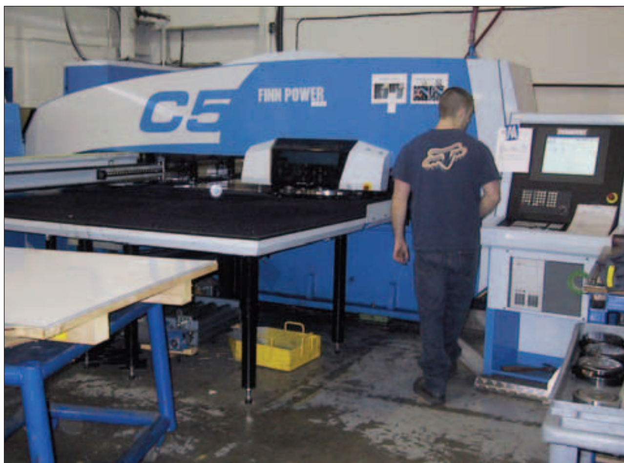
The C5 turret punch press from Finn-Power shown here has helped Wesgar to increase capacity and throughput significantly.
