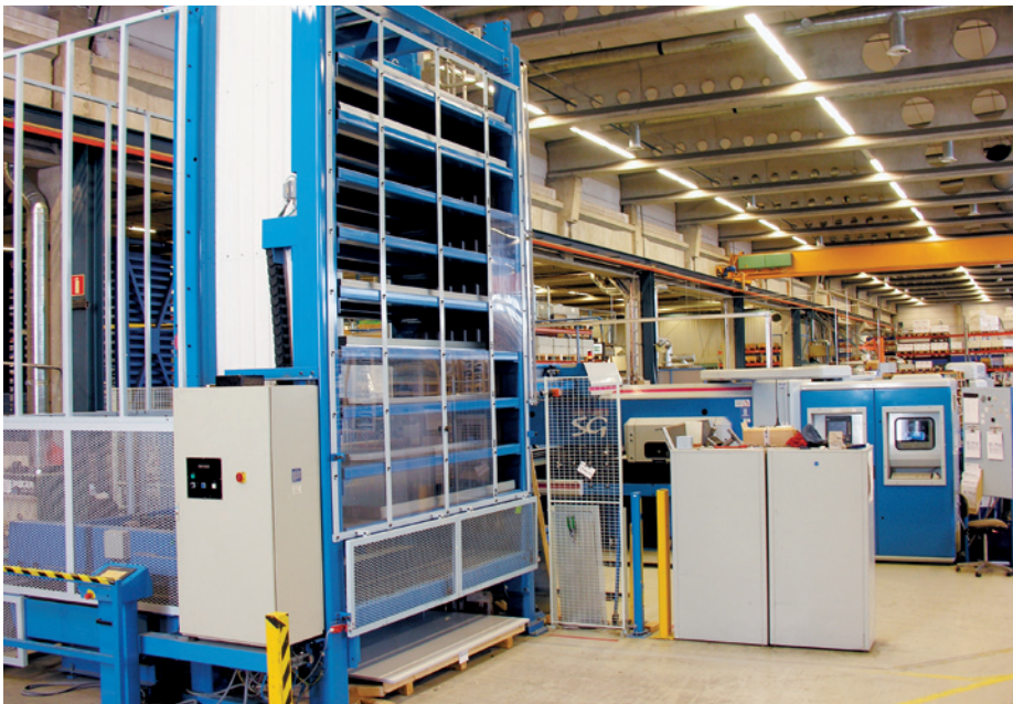
Halton Indoors (Kausala, Finland) fabricates mainly 22 ga. pre-coated sheet steel. The raw material is stored and automatically fed from a computer-controlled Finn-Power Night Train flexible manufacturing system (FMS).
