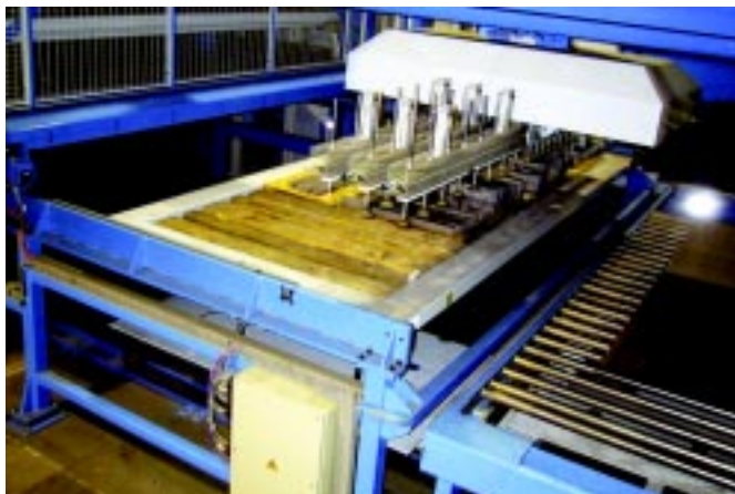
A computer-controlled material handling device is common in highly productive European fabricating operations. These vacuum-operated devices move material from storage or production buffer to machine stations and remove skeletons.
