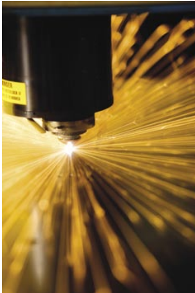
Clean cuts delivered by laser cutting eliminate secondary sheet metal operations common to cutting with a turret punch press.
