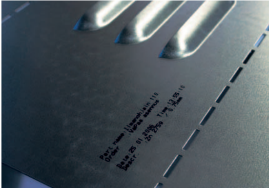
Fast, reliable component marking is a major benefit in JIT manufacturing and subcontracting
