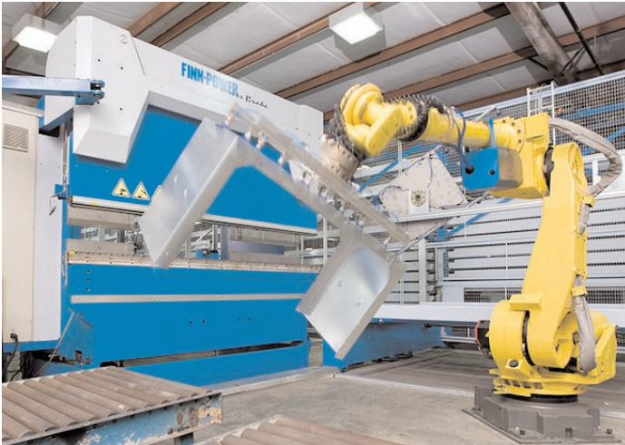
▲ Industrial robots are helpful in eliminating the hazards associated with handling large, cumbersome parts.
