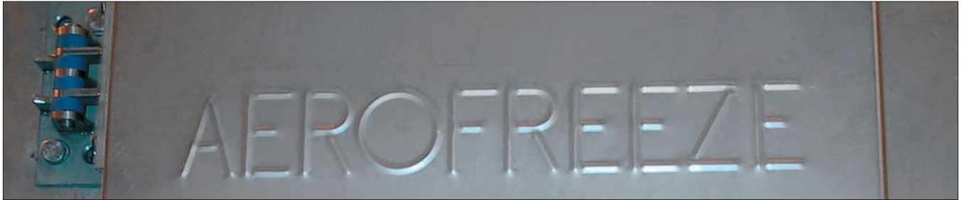
The Aero-heat logo was produced using wheel technology tooling/roller ball. Prior to purchasing the Shear Genius, this part was manufactured as a secondary operation with a separate name plate.
