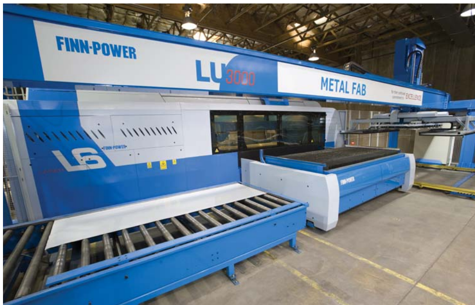
The L6 uses digitally controlled linear drive motor technology for high-speed operation, high acceleration and contour accuracy.
