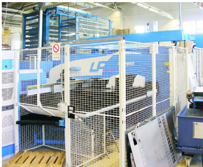
▲ Electronics contract manufacturer InCap installed this laser/punch combination machine in 2005 and a punching/shearing cell with an FMS for raw material and work-in-process this year. Plans call for integrating the equipment into one automated sheet metal fabricating line.
