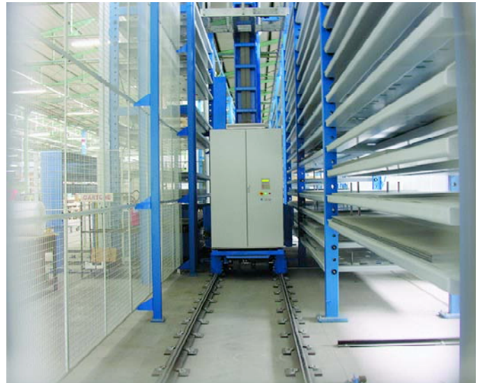
▲ Costan has two Night Train FMSs that, if placed next to each other, are longer than a football field.
