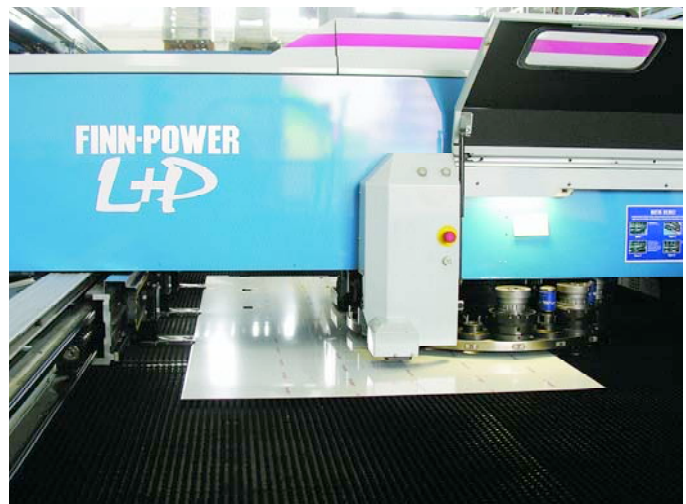
▲ The punching tools on Ilinox's laser/punch combination machine are put to good use creating openings in this cabinet component.
