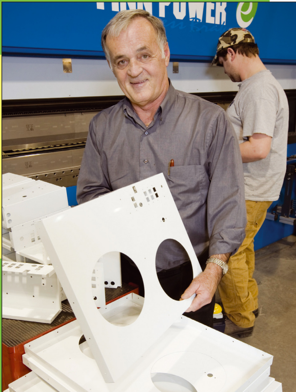
Earl Caldwell says the Shear Genius punch/shear manufacturing cell has cut processing time by two thirds, "huge savings."
