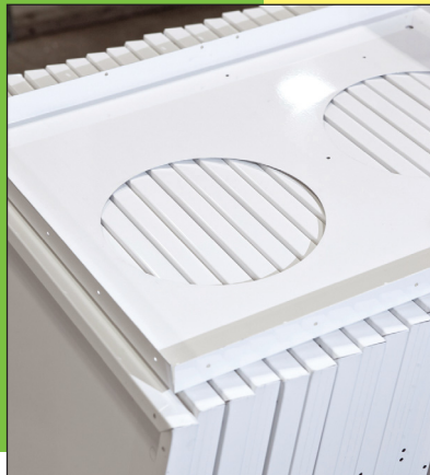
Above: Components of Nu-Air's AIMS product produced on the Finn-Power Shear Genius cell, seen assembled at left.
