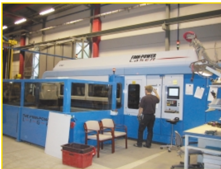
At Halton Marine, linear motor drives position the x/y axes at 11,811 ipm for laser cutting 1-mm stainless steel for range hoods in the galleys of cruise ships.
