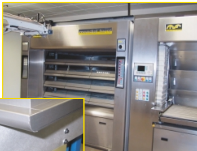
Intricately curved stainless steel panels (inset) are formed without special tooling for bakery ovens at Mondial Forni on a Night Train FMS cell that comprises Finn-Power's Bending Automation and a Shear Genius machine.
