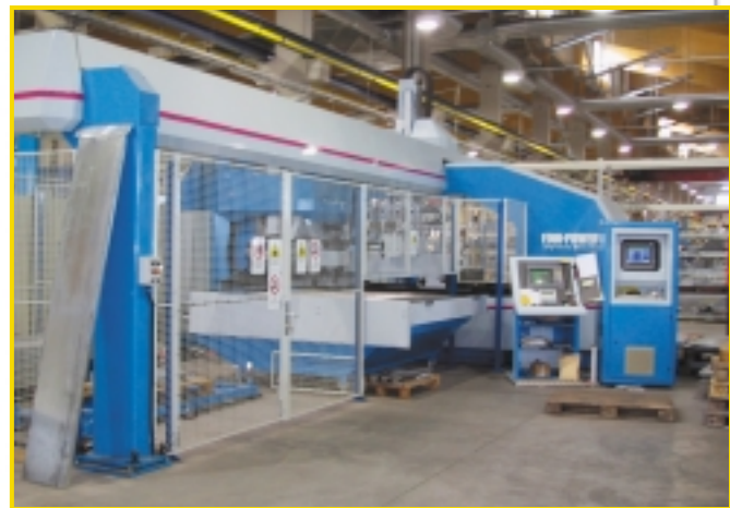
Bottom: At Koja Ltd, the Finn-Power Express Bender uses its unique manipulator to work the edges of the panel, starting at the external edge of the sheet and indexing each side in sequence until all bends are completed.
