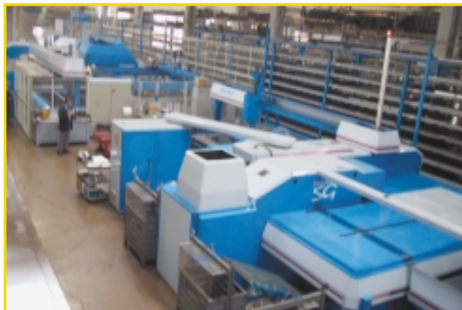
Top: The Night Train FMS cell at Mondial Forni with Shear Genius with special enclosure in foreground and Bending Automation machine.
