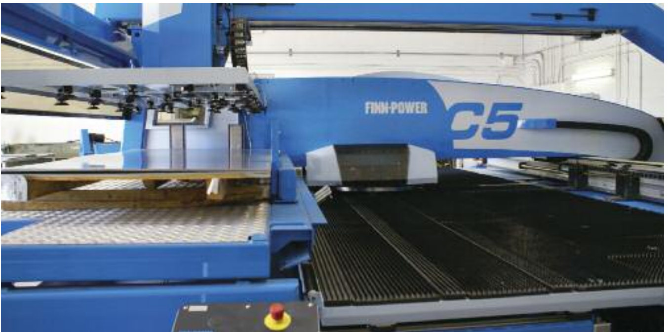
A-G Body employs the automatic sheet loader on its C5 CNC turret punch press for about 75 percent of the work the machine processes, freeing up the machine operator to perform other tasks around the firm's small sheetmetal shop.
